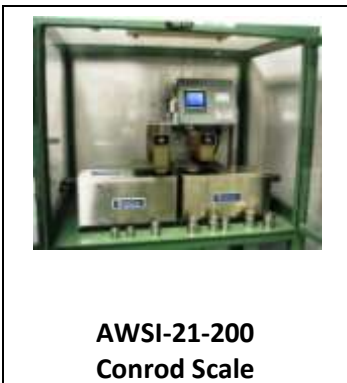
AWSI-200 Weigh-Cell Fast: 125 ms Settling Time Capacities Starting at 300 grams
